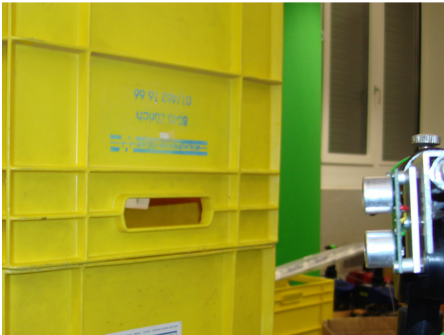
Figure 4.11: The setup to test scenarios C and D. The sensor is mounted on a stand and can be turned toward a pile of plastic cases (yellow).
