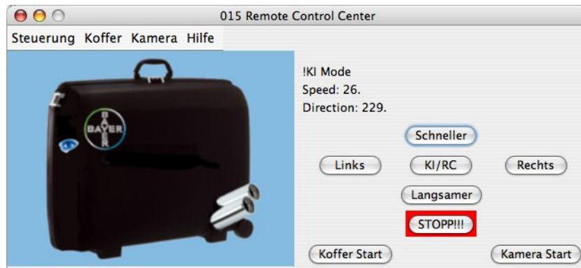
Figure 5.1: The new GUI of the Null15AIControl, that provides access to the robots functionality for the user.
