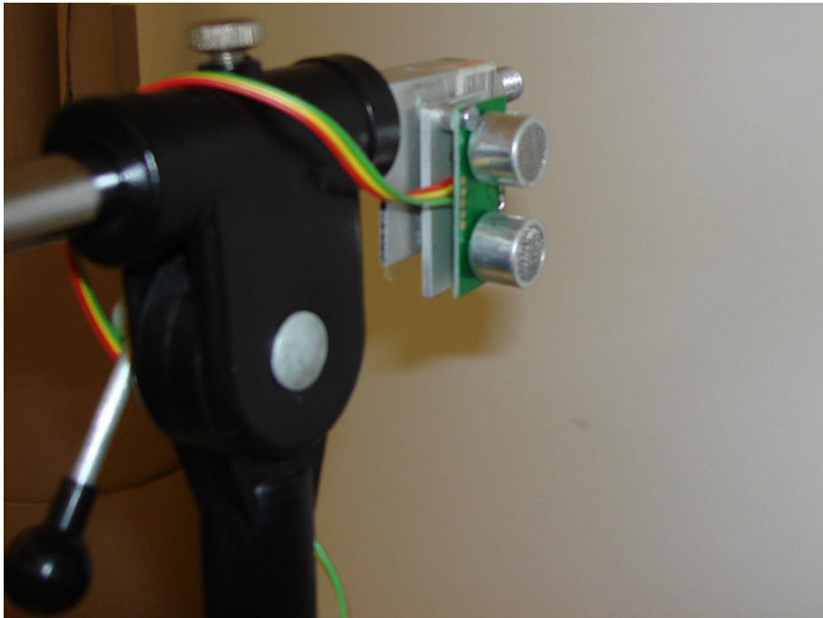
Figure 4.10: The setup to test the scenarios A and B. By turning the sensor toward the wall in the background, the angle can be determined.
