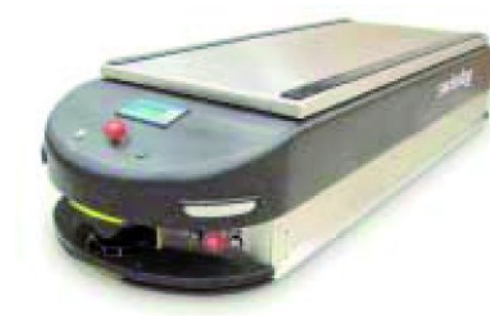
Figure 2.3: The cart of the Swisslog TransCar automatic guided vehicle system.
